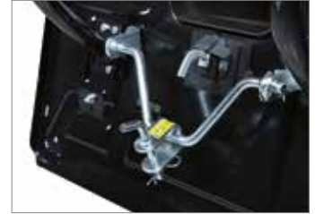
The towing hitch, fitted as standard, makes the machine even more versatile, allowing it to tow a trailer or lawn roller (103).
