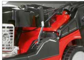
Centralised cutting height adjustment by means of a practical lever with preset positions.
