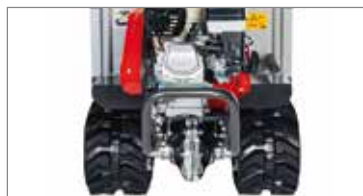
Rear metal guard to maximize operator safety.
