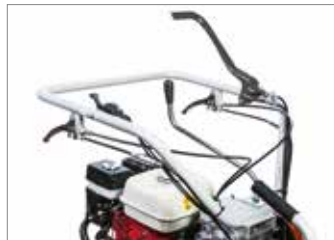
Steering with independently controlled release and brakes.
