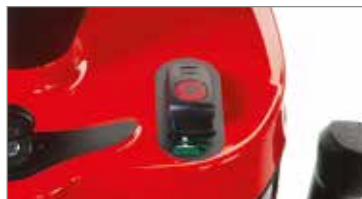
The electromagnetic clutch engages quickly and quietly by way of a handy dash-mounted button.
